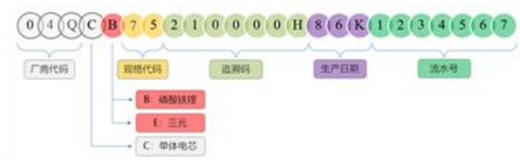
Fig.6 Schematic diagram of QR code knot
