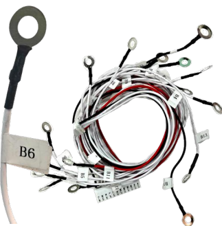
Each wire has a corresponding label
